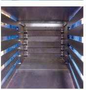
Wear resistant, replaceable Nylatron liners on the ram slides. 500 Brinell steel liners on the floor and ram bottom. Oversized ram hold-down bars are adjustable from the exterior of the machine.
