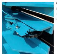
Spring loaded counter wheel, located on the side of the baler, sends a digital reading to the operator interface.
