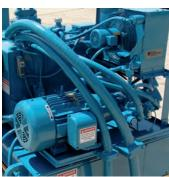
TEFC motor with quiet running pump system.
