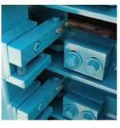
Spring loaded retainer locks, adjustable wire positioners, and adjustable inserter needle positioners.
