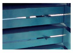
Spring loaded container dogs are located on each side of the bale chamber to produce superior spring back control of materials being processed.
