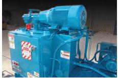
Marathon's advanced power pack is designed so that all the valves are contained in a single manifold, which minimizes the number of hose connections.
