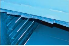
Bolt-on adjustable and replaceable shear blades cut material as a bale is made and minimize problems associated with irregular bales sizes. This makes bales easier to tie and stack.
