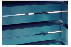
Spring loaded container dogs are located on each side of the bale chamber to produce superior spring back control of materials being processed.
