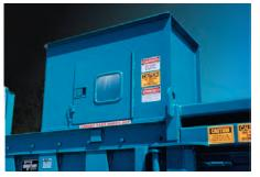
The chute feed hopper with inspection door and interlock switch will accommodate pneumatic, gravity, or conveyor feeding systems.
