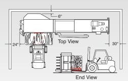
Install Marathon's Side-Eject Baler against a wall or in a tight space. Minimal floor space is needed for operation due to the unique front baler tie-off feature and side-eject design.
