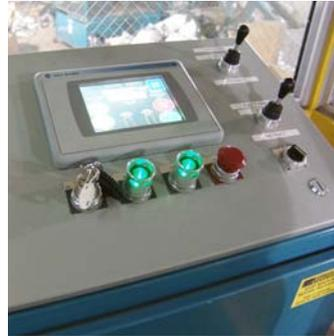
Maestro™ color touch-screen operator interface PLC programmable controller features automatic and manual controls, diagnostics and bale set-up functions. Available with multi-language function.
