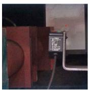
The main ram, ejector ram, and multi-purpose door are controlled by a long range laser sensor. Tie positioning is determined by the laser and eliminates the need for a counter wheel.
