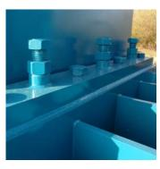
The Galaxy2R® narrow model features an adjustable shear beam that enables you to adjust the shear blades from the exterior of the machine.
