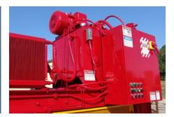
High-efficiency power unit and electrical disconnect.
