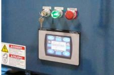
The touchscreen enables full automatic and manual control with one touch. Screens may be customized, password protected, and are designed with alarm, diagnostic, and help screens.
