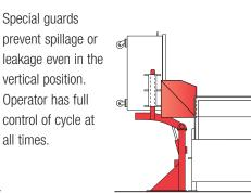
Container is tilted a full 45 degrees past vertical, assuring complete cleanout. Dumping cycle is 26 seconds for the heavyduty and 36 seconds for standard models.
