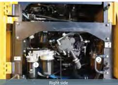
1 Engine oil filter 2 Fuel filter with Water separator
