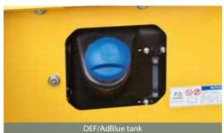
Located inside the standard machine storage compartment
