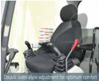
Double slides allow adjustment for optimum comfort
