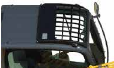
Standard FOPS, Top Guard Level II. (Meets ISO10262)
