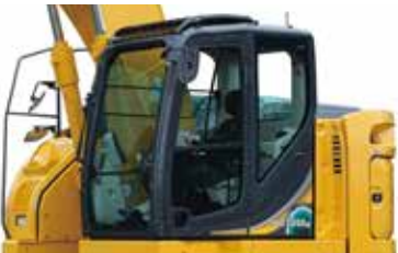
Mounting brackets for vandalism guards are standard equipment (contact your KOBELCO dealer to fit vandalism or front rock guards).
