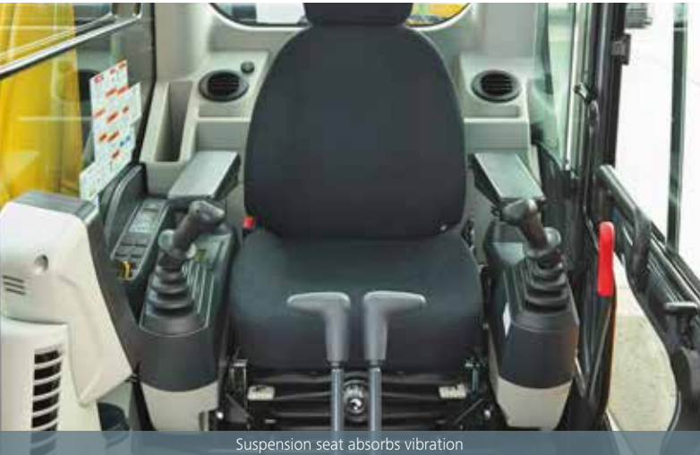
Suspension seat absorbs vibration
