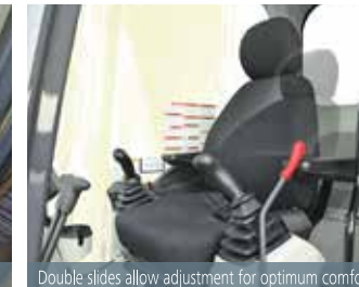
Double slides allow adjustment for optimum comfort
