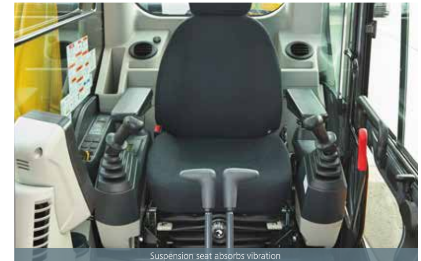
Suspension seat absorbs vibration
