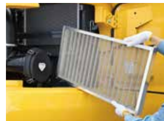
iNDr filter/radiator reservoir tank/air cleaner access.
