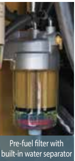
Pre-fuel filter with built-in water separator
