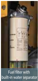
Fuel filter with built-in water separator
