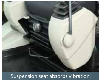
Suspension seat absorbs vibration
