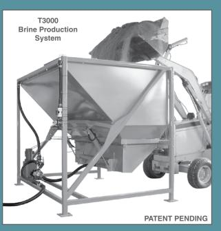
Back View: Heavy Duty Skid Frame (3" Stainless Structural Square Tubing) can be moved easily by a loader with forks or lifted.
