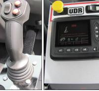
Joystick, mounted in the armrest of the truck for easy access, controls the boom direction, speed, engine throttle and box container dump.
