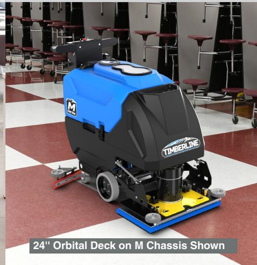
24" Orbital Deck on M Chassis Shown
