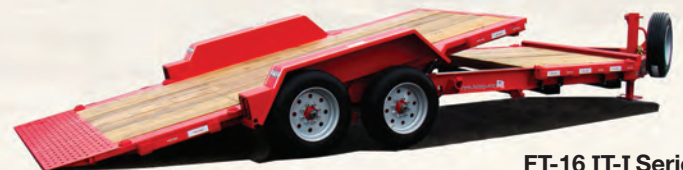
FT-16 IT-I Series (Option: Toolbox, Stationary Platform, Stake & Strap, Fork Pockets, Spare Wheel & Tire Mounted) 80543-LAE
