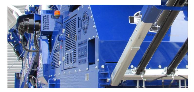
The EDGE LTS 360° Unlimited Range incorporates all the benefits of the popular LTS Series product line and adds an additional design feature, with its ability to slew a complete 360° uninterrupted. Mounted on a centre slew bearing chassis the LTS 360 slewing stockpiler has brought production efficiency improvements in many ports and quarries throughout the globe.
