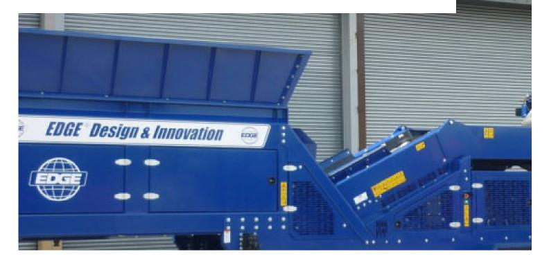
The EDGE FMS mobile hopper feeder is designed for operators who either require a controlled flow of material output or need to feed directly using an excavator or wheel loader. Incorporating a high torque variable speed feed conveyor and various discharge conveyor lengths ranging from 30ft to 75ft, EDGE's mobile feed stockpilers effectively eliminates the need to have both a separate hopper feed unit and a stacker unit.
