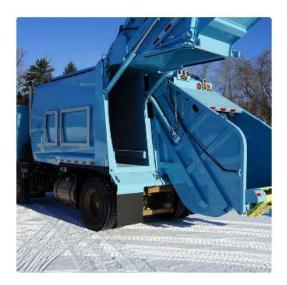
The Enviromaster provides a simple single tailgate solution for your dual stream needs. Designed with a single tailgate with a division in the middle allowing for a lighter less expensive solution that also allows the use of commercial container lifting.
