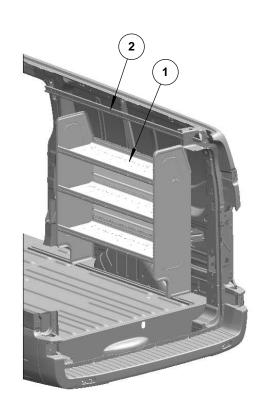
**CAUTION:** DRILL THRU FLOOR WITH CARE! WATCH FOR GAS TANK, CONTROL LINES, & ELECTRICAL WIRING.
