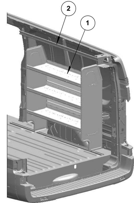
**CAUTION:** DRILL THRU FLOOR WITH CARE! WATCH FOR GAS TANK, CONTROL LINES, & ELECTRICAL WIRING.
