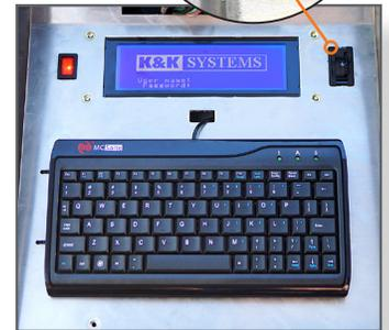
**K&K Systems' Quick Message Selection Thumbwheel** switches between the first 16 user defined messages. Roll the thumbwheel to desired message number to display a message.
