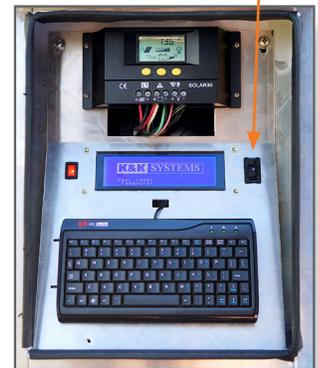
K&K Systems' **Quick Message Selection Thumbwheel** switches between the first 16 user defined messages. Roll the thumbwheel to desired message number to display a message.
