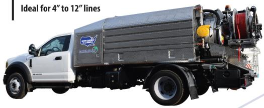
STAINLESS STEEL CONSTRUCTION: Debris tank, water tank, hose reel and full shroud
