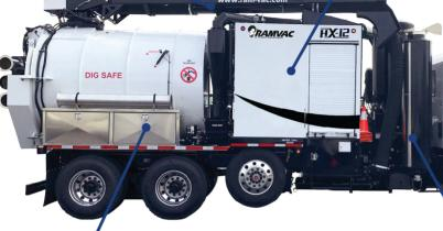
RAMVAC HX trucks come standard with locking differentials and power diverters to help you get out of the most difficult terrain. Its design ensures one of the smallest footprints in the industry, allowing you to get into those tight spots where other hydro excavators will not fit.
