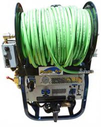
12 GPM @ 3000 PSI Sewer Jetter
