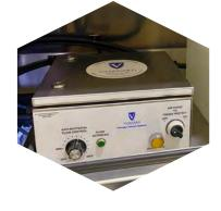
1. Control box automatically meters and blends Sani-Solution™ concentrate with on-board water.
