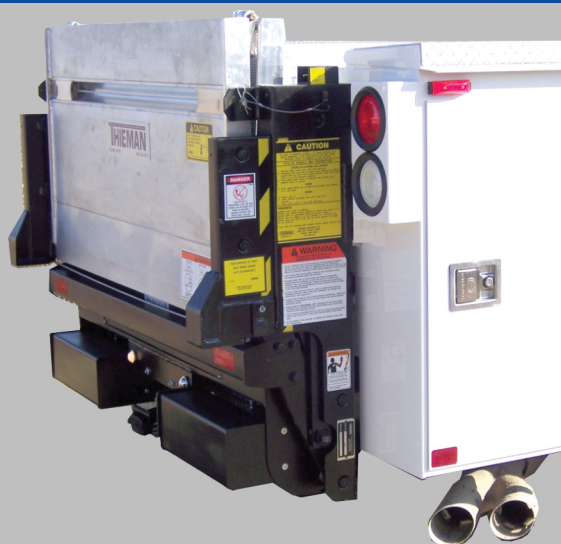
Shown with Optional Two-Piece Alum. Platform
