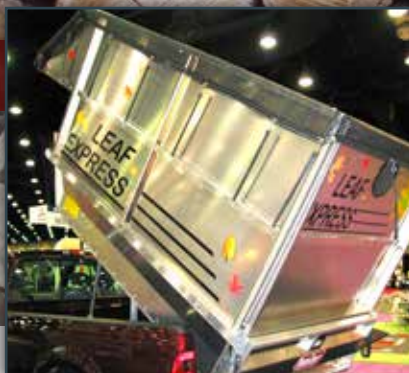
TC-150 Leaf Express. All aluminum leaf topper fits on TC-121 and adds 7.6 cu. yds. of volume. Comes in tarp-top or hardtop version. Weighs less than 300 lbs. One year wty.
