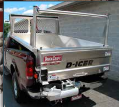
TC-131 D-ICER all aluminum and stainless steel tailgate replacement salt spreader. Spreads 10,000 lb/hr.
