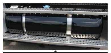
Pac-Mac can accommodate a variety of CNG tank options including saddle tanks below the rail or back of cab, above the rail
