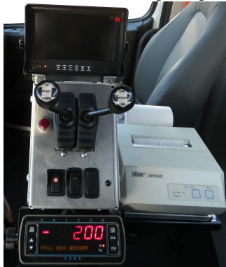
*Patent Pending ergonomic control console that includes: rear camera monitor, hoist controls, work lights switch, PTO switch, and optional on-board scale digital read out and printer.
