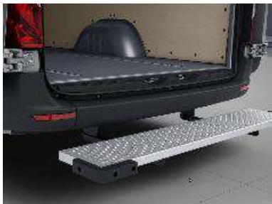
The code W75 includes a hot-dip-galvanized steel step fitted at the rear of the vehicle. The step measures 63 x 11,81" (1,600 x 300 mm) (width x depth). Solid rubber mouldings on the outer corners provide protection when manoeuvring.
