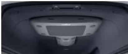
The rear air conditioning system is mounted onto the rear part of the roof and partially on the inside roof of the vehicle that comfortably cools the rear compartment. Compared to MY18 the roof unit is located more towards the rear of the vehicle.
