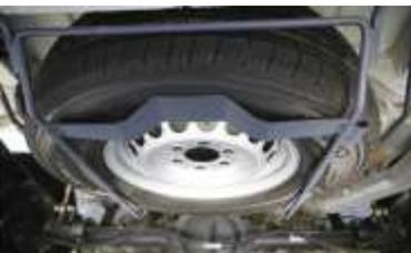
The spare wheel bracket is mounted under the end of the frame behind the rear axle.
