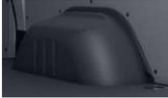
The code V35 includes black rubber covers for the wheel housings, protects them from damage, and provides additional noise insulation.
