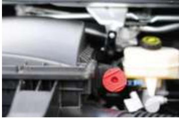
A jump-starting connection point is located on the air filter box in the engine compartment and allows easier jump starting or charging of the starter battery. The terminal can be accessed by pushing back the red protective cap for the positive terminal and a brass rod on the inner left fender for ground.
