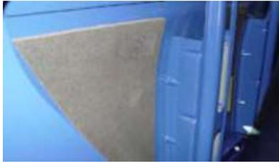
Insulation material is fitted up to the belt rail in the sidewalls of the load/passenger compartment and in the rear doors.
