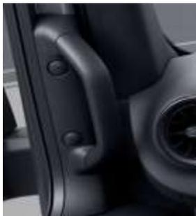
The grab handle is installed vertically on the driver and passenger door of the vehicle, and facilitates getting into the vehicle providing another option to hold on the way.
