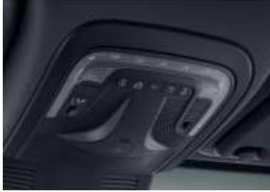
The Overhead Control Panel with interior lighting control, Code L1D, is comparable to the Comfort overhead control panel but includes an additional button to operate a retrofitted interior lighting for buses. The interior lighting in the rear is dimmed when activated.
