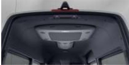
The rear air conditioning system is mounted onto the rear part of the roof and partially on the inside roof of the vehicle that comfortably cool the rear compartment.
