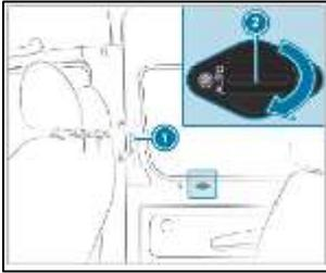
The opening limiter is a fixed stop of the sliding door at an opening of 30.7” (780 mm). This allows passengers a faster step in and out of the vehicle.
