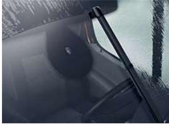
The code JF1, Rain sensor, automatically regulates the activity of the wind-screen wiper when set to interval. It is located centrally at the top behind the wind screen and registers wetness levels on the sensor surface. The rain sensor can be set to two different wiping speeds and the sensitivity of both settings can be further differentiated.
