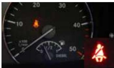
An optical signal in the instrument cluster reminds the driver to buckle up when starting the vehicle. If this is ignored and the vehicle is in motion 15 mph (25 km/h) an acoustic signal sounds.
