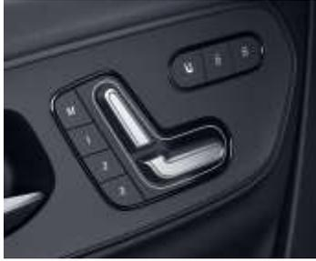
This electrical driver seat is based on the driver's comfort seat code SB1 and has the same adjustment options. The main difference is the head restraint height and seat cushion length. All adjustments can be made electrically using the switches on the control unit located on the driver's door.
