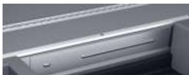
When ordering this code an aluminum strip is mounted to the wooden floor in the entrance area of the right load compartment sliding door. In order to make the strip fit perfectly that part of the wooden floor is milled out and the aluminum strip inserted into the recess. The strip serves to protect the edge of the floor from damage when entering and exiting, or loading and unloading.
