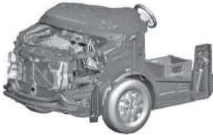
The cowl platform, is based on the cab chassis but without a windshield, roof frame, rear wall and doors. This type of vehicle provides upfitters a basis for fitting fully integrated superstructures e.g. campers or special-purpose solutions. The cowl version comes always without a driver and co-driver's airbag. Comfort seats with swivel base for driver and passenger are part of the vehicle configuration.
