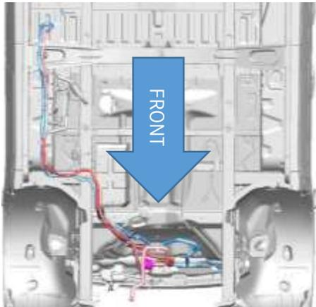
Two water lines (supply line/return line) are routed under the floor panel on the left-hand side of the vehicle, extending after the B-pillar. The ends of the two lines are connected by a hose. This allows an easier fitting of aux. heater exchanger from the accessories range. The opening in the floor (cargo/passenger van) /wooden floor for the warm air ducting and electrical parts e.g. climate control panel, wiring harness are not included.
