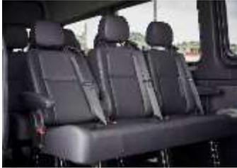
A three-seater comfort bench is fitted in the **first** row of the 14+1 passenger compartment. All three seats are fitted with a three-point seat belt and have additional seat bolster padding, allowing for enhanced seating comfort. This comfort variant can be equipped on Crew and Passenger Sprinters. Each row is individually reclinable as well as an individual recliner setting on each seat.
