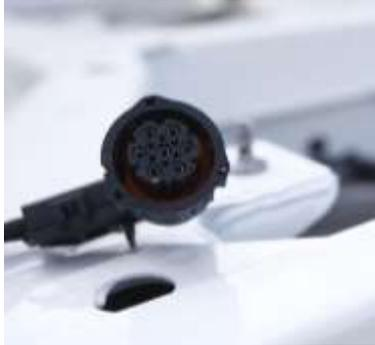
Wiring for trailer hitch that runs along the inside left frame. E40 includes a seven-pin connector and provides power for trailer lightning systems (tail lights, brake lights, direction indicators, rear fog lights and reversing light) and allows electrical operation. The trailer wiring is bundled up and temporarily attached to the frame during transport. This allows for installation of an authorized accessory trailer hitch by the body builder.
