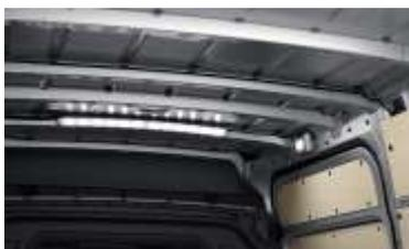
In addition to the standard interior lighting, two LED lights approximately 30" (762 mm) long (3000 K, warm white, approx. 20 Lux; luminous flux: approx. 400 Lumen) are included. These are located in the center of the entry area and on the back roof bow of the load compartment. The lights can be switched on and off either using the interior-light switch by the rear door via the door contact switch or via an overhead control panel with switch for interior lighting in the rear.
