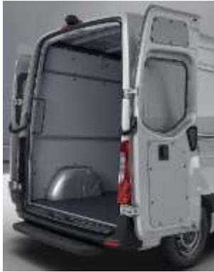
With W54, hinges are installed that allow the rear doors to be opened to the side wall of the vehicle. The new hinges hold the doors in place on its own without the need of rubber, magnetic bumpers on the door/side wall. This makes loading much easier in confined spaces, for example on ramps. The newly developed door hinges engage automatically at 90° and in the maximum opening position.
