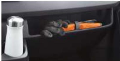
An open storage compartment is included on the co-driver's side. The dimensions of the storage compartment are 18.9 x 3.94 x 6.3" (480 x 100 x 160 mm) (Width x Height x Depth). FJ4 replaces the former lockable glove compartment.
