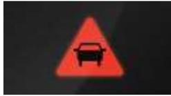
The Active Brake Assist with cross traffic function continuously checks for a safe distance of the vehicle in front and warns the driver both optically and acoustically of potential collisions (e.g. rear-end collision) with other vehicles, significantly reducing the risk of accident.
