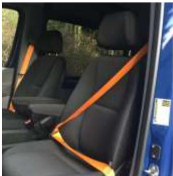
Orange safety belts replace the standard black safety belts for the driver and passenger (not with S23, twin passenger seat).
