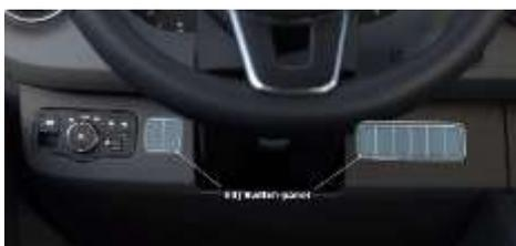
This pre-installation includes two additional switch panels below the steering wheel with a total of eight possible switches, where two switches are located to the left and six switches are located to the right. The covers can be exchanged in the future to functioning switches for retrofitting purposes.
