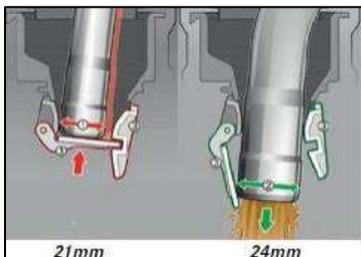
The protection system is designed for diesel models and includes a locking device with two levers that is made in such a way that it can only be unlocked by a standardized diesel pump nozzle. This prevents the tank from inadvertently being filled with gas. The diameter of the standardized gas pump nozzle (0.83" (21 mm)) is smaller than the diesel analogue (0.94" (24 mm)) and therefore too small to unlock the mechanism.
