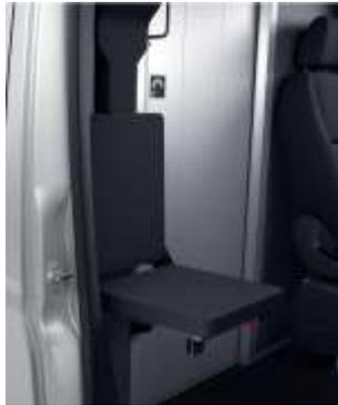
The foldable co-driver seat and its head restraint are directly attached to the partition with sliding door. This seat makes it easier for the driver to enter or exit the vehicle on the passenger’s side and provides easier access from the passenger door into the load department. The upholstery is always fabric maturin black without any sales code. For folding the seat cushion up or down the red button needs to be pushed first.
