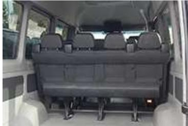
A four-seater comfort bench is fitted in the **third** row of the passenger compartment. All four seats are fitted with a three-point seat belt and have additional seat bolster padding, allowing for enhanced seating comfort.
