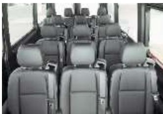
The 14+1 seater version, with four rows of seat benches, is for the passenger van (BM907.745) with weight variant of 9,480lbs (4,300kg). All benches include three-point seat belts and can be upgraded with available comfort packages and options.
