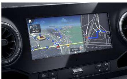
With this, the MBUX multimedia system with 7" touch display (code E3M) becomes a full-fledged navigation system including free map data updates for 3 years. It can be operated either via touch screen, the buttons on the control unit below the touch screen, or via touch-control buttons to the right of the multi-functional steering wheel. Navigation can be displayed both on the display of the multimedia systems and the instrument cluster. This is not available on the 10" MBUX multimedia system
