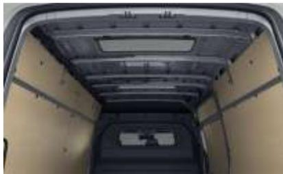
The 144" WB vehicles are with two fixed sunroofs that are installed in the front and rear sections of the load compartment. The dimensions of each sunroof are about 32.68" x 15.75" (830 x 400 mm). The 170" WB vehicles and 170" WB Ext. vehicles are fitted with the two sunroofs mentioned above, and two additional fixed sunroofs in the rear section of the roof (dimension approx. 6.69" x 20.47" (170 x 520 mm))
