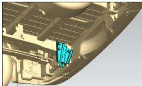
Reinforcements are welded to both rear left and right longitudinal members where these inserts serve an additional base for different options, such as trailer couplings, steps and cross members.
