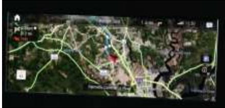
This replaces the previous generation ‘Intelligent Navigation’ (E1G). The communication module forwards the real-time traffic data to the head unit and receives position data from the head unit at regular intervals in the opposite direction. The position data is sent to the service provider. The HERMES control unit therefore contributes to collecting the traffic information from
