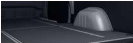
The code V43, wood flooring, includes a plywood floor installed in the load compartment. The top of the wooden floor is coated with a grey, hardwearing and non-slip melamine resin film. The bolted lashing points fix the wooden floor down. The number of anchoring lugs utilized varies according to the length of vehicle.
