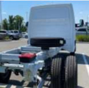
All vehicles come with the spare wheel bracket mounted under the end of the frame which allows to carry a full-sized spare wheel (except the super single). For cab chassis where the area of the rear frame end is used for custom upfits, the spare wheel can be provisionally mounted on the frame via code R60. In this case the spare tire must subsequently be relocated to another position in or on the vehicle.
