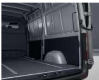
The side walls and doors of the passenger/load compartment are covered with 0.08" (2.03 mm) thick black wood-dust filled polypropylene boards from floor up to the height of the window sill girder, code V25. The wood-dust filled polypropylene boards are hydrophobic, washable, robust and 100 % recyclable.
