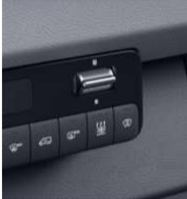
In addition to the heater booster, with the auxiliary hot-water heater, the departure time can be programmed in the instrument cluster using the stationary heater button in the climate control panel on the multi steering wheel.
