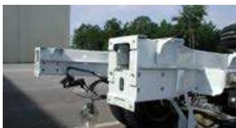
The rear end cross member is not fitted. Four weld nuts are fitted at the mounting plate corners.
