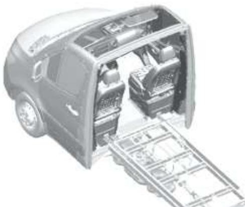
Chassis without rear wall and roof, but including seat bases. A cover (code P08) is supplied for transport purposes.
