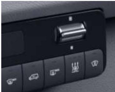
Windows with heating filaments are fitted in the rear doors. The rear window heating function is switched on by a switch with integral indicator light. The rear window heating function can only be switched on when the engine is running. It switches off automatically after approximately 5 minutes, or can also be switched off manually
