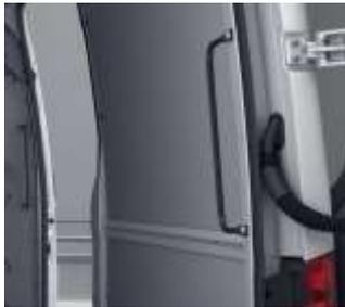
This grab handle(s) is installed vertically on the right D-pillar and allows an easier entry to the load compartment through the rear door.
