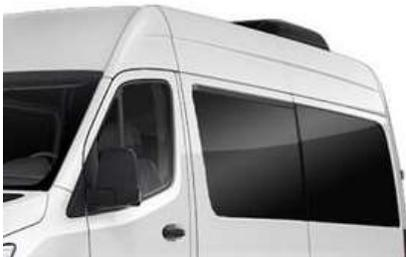
Laminated glass is installed for the side windows behind the driver/passenger and –if applicable- behind the last seat row. It is a legal requirement (FMVSS 226) for vehicles with a gross vehicle weight rating (GVWR) of up to 10,000 lbs. without a partition wall and this is met.
