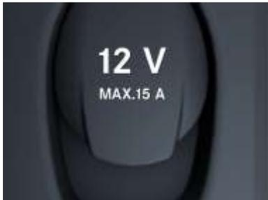
A 12 V / 15 A socket with a maximum power consumption of 180 W is installed on inner side of the driver ´s seat frame. The socket is supplied with power by the starter battery, except if code E2I/E2M is ordered, and then it is supplied by the auxiliary battery. In this case, power can be drawn regardless of ignition status.
