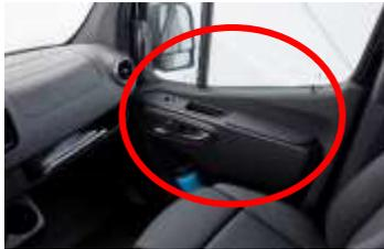
The cushioned armrests on the driver's and co-driver's door, code S28, are optionally available. The faux-leather armrests offer an increased level of comfort and are mounted behind the door switch and handle.
