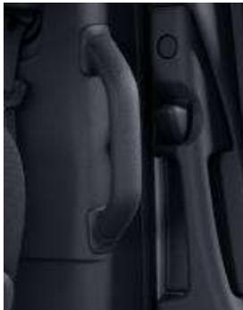
This grab handle(s) is installed vertically on each B-pillar if the vehicle is equipped with sliding door(s) and allows an easier entry to the load/passenger compartment through the sliding door(s).
