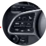
The cruise control accelerates and brakes the vehicle automatically in order to maintain a previously stored speed above 15 mph (24 km/h). The cruise control is operated using the left steering wheel buttons. A limiter function is not available. If the cruise control is activated and the optimal available Traffic Sign Assist has detected a speed restriction sign, the maximum permissible speed displayed in the instrument display can be stored
