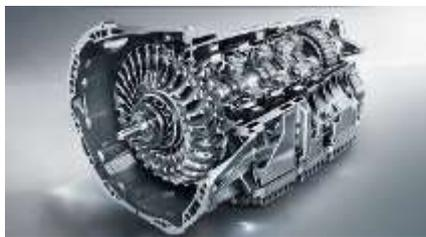
**The Automatic Transmission 9G-TRONIC** is fully electronically controlled with nine forward gears and one reverse gear. The gear ratios for the gear ranges are realized with planetary gear sets. All transmission functions and components are combined in one assembly module. The fully integrated transmission controller unit is located in the automatic transmission. This minimizes the number of interfaces to the vehicle wiring harness.
