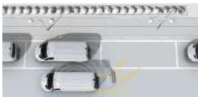
The parking system is using twelve distance sensors and the reversing camera. It supports the driver during the parking procedure, when maneuvering in confined spaces and when driving out of exits.
