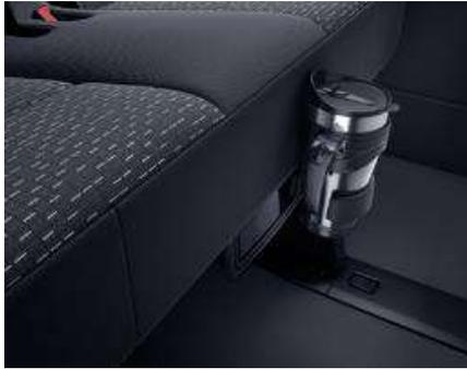
Cup holders are mounted between the rear seats on each bench. One cup holder can carry two cups or bottles with a diameter of up to 3.3" (84 mm). The cup holders can be ejected individually by pushing on its flap.
