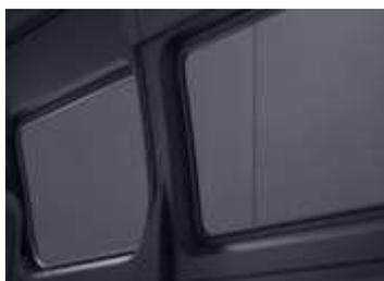
The standard painted window pillars can be lined, between the roof trim and the side trim, with matt black washable plastic paneling.
