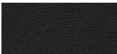
Seat cushion, back rest, seat bolsters, head rest and the back of the seat are covered in artificial leather. However, the seat bolsters (seat cushion only) of the driver's seat are covered in real leather. The low-wear artificial leather is easy to clean using water and a suitable soap-based detergent.
