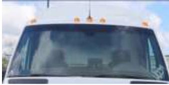
Vehicle marker and clearance lamps are required by law on all vehicles with a total width of 80" (203 cm) and above according to FMVSS standards. The five identification lamps are mounted in the area of the windshield at the vehicle roof. The two outer ones are used as clearance lamps and the three inner ones are identification lamps. The preparation clearance lights includes the wiring harness (tied in the roof) and allows an easier installation of the lights on the roof.
