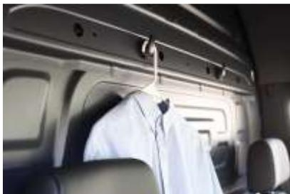
The two coat hooks in the cab are available for the cargo van and mounted above the head restraints on the partition wall inside of the driver’s and co-driver’s seats.
