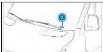
The code XC8 includes a VIN-plate (Vehicle Identification Number) affixed on the left side of the dashboard underneath the windshield what is visible from the outside.
