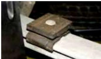
Installation of two vibration dampers each on the left and right rear spring. Rubber absorbers providing optimal vibration damping and reducing noise levels in the vehicle
