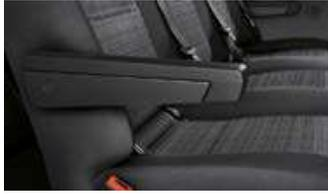
An arm rest is fitted to the aisle side of the backrest of the passenger bench seat, allowing for enhanced seating comfort.
