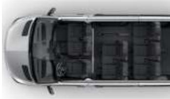
A three-seater bench is fitted in the **second** row of the passenger compartment. All three seats are fitted with three-point inertia-reel seat belts. ISOFIX child seat attachment points are on the two outer seats.
