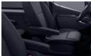
A tilt-adjustable armrest is fitted to the inboard side of the driver’s backrest. Retrofitting this armrest entails swapping the entire backrest.
