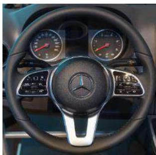
The multifunctional steering wheel allows for the driver to operate the on-board computer, vehicle functions, and multimedia systems without taking their hands off the steering wheel. This is done via touch-control and push buttons.
