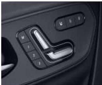
This electrical passenger seat is based on the driver's comfort seat code SB2 and has the same adjustment options. The main difference is the head restraint height and seat cushion length. All adjustments can be made electrically using the switches on the control unit located on the co-driver's door.
