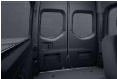
The luxury interior paneling, code V21, in dark grey fabric gives the passenger compartment a representative look, and also improves the noise and heat insulation. The paneling is made of wood-dust filled polypropylene boards and a 0.12" (3.05 mm) thick layer of polyurethane foam, all lined with fabric. This paneling includes 5V USB-C charging ports with a smart phone holder for each row installed on the left side of the vehicle.
