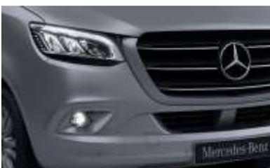
The halogen front fog lamps are integrated into the front bumper and support a cornering light function whereby one of the two front fog lamps switches on automatically when the driver activates a direction indicator or turns the steering wheel. The cornering light dims on at speeds up to 25 mph (40 km/h). A curve light function dims on at speeds up to 43 mph (70 km/h). The fog lamps can be switched on/off with a button at the light switch positioned on the
