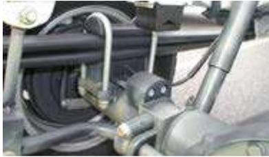
This includes shock absorbers tuned specifically for passenger transport as well as additional springs and rubber bearings compared to the base suspension. It additionally has an application of double-leaf parabolic springs with progressive spring characteristic which increase the driving comfort in unloaded vehicles. The spring is designed to be “soft” under low applied force, and becomes “firmer” when the vehicle is loaded, ensuring suitably firm
