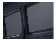
The standard painted window pillars can be lined, between the roof trim and the side trim, with matt black washable plastic paneling.
