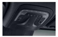
The emergency call system allows a manual, via the SOS button, or automatic emergency call (when airbags have been deployed) to be triggered. After the emergency call has been triggered, the communication module establishes a connection to the Mercedes-Benz Service Center. If possible, the agent speaks in the language selected in the system settings of the head unit. A microphone is used for the voice input. The communication module relays the incoming voice signals via the center speaker in the
