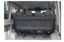
A four-seater <u>comfort</u> bench is fitted in the **third** row of the passenger compartment. All four seats are fitted with a three-point seat belt and have additional seat bolster padding, allowing for enhanced seating comfort.
