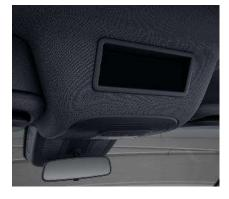
An opening (1 DIN slot) is centrally located in the headliner above the windshield. This slot can be used for additional electronic devices. It comes with a cover for delivery and includes a cable set which reaches into the slot and offer the following connections:
