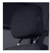
The standard 2-way head restraints of the front seats can be replaced with the comfort variant. The comfort variants are characterized by manually adjustment options:
