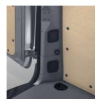
A 12-volt socket is located in the left-hand D-pillar trim of the passenger/cargo Van. The passenger Van also has a 12-volt socket in the right-hand D-pillar trim. Both sockets have a maximum power rating of 180 watts. Power can be drawn regardless of ignition key position. The sockets are supplied with power by the starter battery, except if code E2I/E2M is specified, in which case it is supplied by the auxiliary battery.
