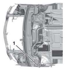
This pre-installation is a standardized interface located in the driver's side A-pillar to easily connect predefined electrical vehicle functions to upfitter devices. It includes 12 upfitter special signals:
