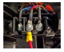
The terminal strip is installed inside the driver seat frame, allows easy integration of additional electrical consumers into the existing network, and offers three connectors:
