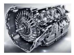
The Automatic Transmission 9G-TRONIC PLUS replaces the 7G-TRONIC PLUS (G42) transmission. It is fully controlled electronically with nine forward gears and one reverse gear. The gear ratios for the gear ranges are actuated with planetary gear sets. All transmission functions and components are combined in to one assembly module. The fully integrated transmission control unit is located in the automatic transmission. This minimizes the number of interfaces to the vehicle wiring harness.
