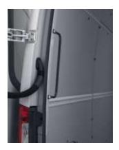
This grab handle(s) is installed vertically on the left D-pillar and allows an easier entry to the load compartment through the rear door.
