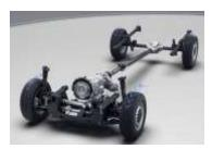
The new <u>all-wheel drive</u> is available with the 2500/3500XD Sprinter as a cargo and crew, with the 2500 as a passenger and with the 3500XD as a cab chassis. This is only available with code M5N, OM654, 4 cyl D-High out (211 hp). The system is "ALWAYS ON" and is in RWD (when driving under normal conditions) but can distribute up to 50% torque to the front axle, if needed. There is no switch to activate the system and thus no indication on the instrument cluster that the
