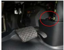
battery master switch is only disconnected when the vehicle key in ignition is in position 0, otherwise there is a risk of damaging other components in the electrical system. The battery quickdisconnect is standard on all Sprinters.
