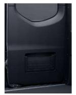
An additional storage compartment with nets is integrated into the door panels of the rear doors. This creates storage facilities for various items, such as Straps or work gloves, directly on the inside of both rear doors.
