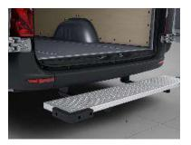
The code W75 includes a hot-dip-galvanized steel step fitted at the rear of the vehicle. The step measures  $63 \times 11,81$ " (1,600 x 300 mm) (width x depth). Solid rubber mouldings on the outer corners provide protection when manoeuvring.
