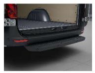
A slip-resistant step is fitted at the rear of the vehicle, extending across the full width of the doors
