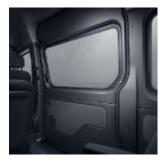
The matte black washable plastic paneling is available for the right-hand sliding door and for the hinged rear doors. This paneling completely covers all metal parts; therefore, improving a visual upgrade of the passenger compartment. In addition, it improves the sound and heat insulation.
