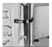
When loading and unloading on an incline or, for example, in strong winds: additional blocks allow the rear doors of the Sprinter to be mechanically fixed at an angle of 90°. This facilitates access to the load compartment and ensures that the rear doors do not close unintentionally.
