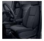
The lumbar support in the backrest of the driver's seat enables the seat to be adjusted to suit the driver's ergonomic comfort requirements. Both air bladders are adjusted pneumatically. The height of the bladders and the extent of the curvature can be controlled with a 4-way switch at the outside of the driver's seat. This optional feature is available for 3 seat variants. Seats fitted with lumbar support meet the criteria of the German AGR campaign for healthy spines.
