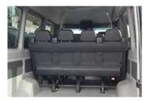
A four-seater <u>comfort</u> bench is fitted in the **fourth** row of the 14+1 passenger compartment. All three seats are fitted with a three-point seat belt and have additional seat bolster padding, allowing for enhanced seating comfort.
