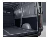
The side walls and doors of the passenger/load compartment are covered with 0.08" (2.03 mm) thick black wood-dust filled polypropylene boards from floor up to the height of the window sill girder, code V25. The wood-dust filled polypropylene boards are hydrophobic, washable, robust and 100 % recyclable.
