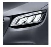
LED High performance headlamps give the vehicle front a high-quality look, the headlamps illuminate the lane evenly both with standard driving light and full beam. The LED technology produces a pleasant soft light from the quantity of light sources, additionally the light distribution is more homogenous compared to the halogen headlamps. Another benefit is the low direct glare for oncoming traffic and other road users. The LED lights also have a long lifespan and consume little power.
