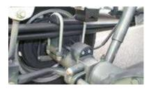
This includes shock absorbers tuned specifically for passenger transport as well as additional springs and rubber bearings compared to the base suspension. It additionally has an application of double-leaf parabolic springs with progressive spring characteristic which increase the driving comfort in unloaded vehicles. The spring is designed to be "soft" under low applied force, and becomes "firmer" when the vehicle is loaded, ensuring suitably firm
