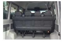
A four-seater bench is installed in the passenger compartment, **third** row. All four seats are fitted with three-point inertia-reel seat belts.
