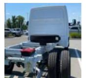
All vehicles come with the spare wheel bracket mounted under the end of the frame which allows to carry a full-sized spare wheel (except the super single). For cab chassis where the area of the rear frame end is used for custom upfits, the spare wheel can be provisionally mounted on the frame via code R60. In this case the spare tire must subsequently be relocated to another position in or on the vehicle.
