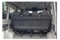
A four-seater bench is fitted in the **fourth** row of the 14+1 passenger compartment. All four seats are fitted with a three-point seat belt and can be upgraded with available packages and options ordered as a comfort variant. (UY6)
