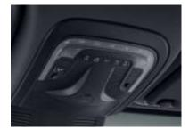
The Overhead Control Panel with interior lighting control, Code L1D, is comparable to the Comfort overhead control panel but includes an additional button to operate a retrofitted interior lighting for busses. The interior lighting in the rear is dimmed when activated.
