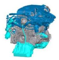
The engine M274 is a 4-cylinder gas engine with an aluminum alloy crank case, direct injection and fast-acting piezo-injectors for multiple injection, needs-orientated multi spark ignition, controlled oil pump, switchable water pump and high compression one-stage turbocharging. Common features are the use of state-of-the art technologies for maximum efficiency, very smooth running, high tractive power right from low revs, sustainability in terms of impending emissions standards and low weight.
