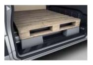
A pallet support is available for the standard step in the load compartment (sliding door). The two plastic inserts are latched onto the step and close the gap between the closed sliding door and the floor of the load compartment.
