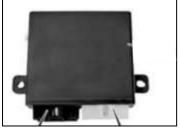
The parameterizable special module (PSM) gives upfitters access to individual types of CAN bus data. The PSM is able to read messages of the various bus data and then, for example, translate them into switching signals at the outputs provided or PWM signals or forward those to a specific body manufacturer upfitter CAN. The installed electronics then have access to the necessary signals.
