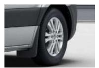
Plastic mud flaps are fitted to the wings behind the front wheels.
