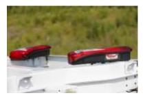
The wiring harness of both tail lights are approx. 78.7" (200 cm) longer than the standard one. They are rolled up and provisionally fastened at the rear frame end and allows upfitters to fit taillights easier in a different position.
