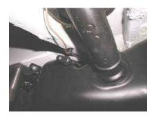
The fuel gauge sensor is fitted with an additional fuel connection to facilitate retrofitting of a fuel-powered auxiliary heater and similar smaller consumers. The fuel tank can be consumed down to approximately five gallons. A "pig tail" (see picture) is located next to the fuel filler pipe and can be easily accessed from the driver side.
