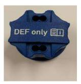
This code includes a blue filler cap for the DEF tank and a plastic key element for diesel engines. To lock or unlock the filler cap the dust protection must be turned to the side and the key element needs to be inserted. This makes it possible to turn and remove the DEF filler cap. After the DEF tank has been filled and closed, the key element can be removed. The key element is with the tool kit enclosed in the storage compartment on the passenger 's foot well.
