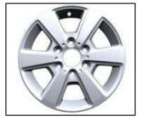
Installation of four 6.5 J  $\times$  16 light-alloy wheels with longer wheel bolts (73 mm) for 235/65 R 16 C tires.
