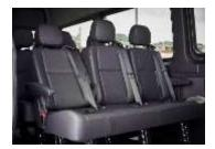
A three-seater <u>comfort</u> bench is fitted in the **second** row of the passenger compartment. All three seats are fitted with a three-point seat belt and have additional seat bolster padding, allowing for enhanced seating comfort. Each row is individually reclinable as well as an individual recliner setting on each seat.
