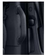
This grab handle(s) is installed vertically on each B-pillar if the vehicle is equipped with sliding door(s) and allows an easier entry to the load/passenger compartment through the sliding door(s).
