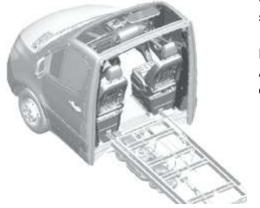
Chassis without rear wall and roof, but including seat bases. A cover (code P08) is supplied for transport purposes.
