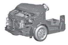
The cowl platform, is based on the cab chassis but without a wind-screen, roof frame, rear wall and doors. This type of vehicle provides upfitters a basis for fitting fully integrated superstructures e.g. campers or special-purpose solutions. The cowl version comes always without a driver and co-driver's airbag. Comfort seats with swivel base for driver and passenger are part of the vehicle configuration.
