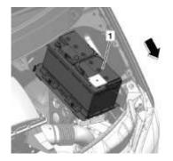
If an installation in the passenger's seat frame is not possible due to upfit restrictions, an additional 12 V / 70 Ah 720 A, AGM battery can be ordered into the engine compartment on the left hand side in driving direction, via code E2M. The battery is ideal for powering additional electrical consumers without putting a load on the starter battery. A cut-off relay (E36) must be ordered with an additional battery.
