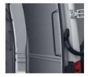
This grab handle(s) is installed vertically on the right D-pillar and allows an easier entry to the load compartment through the rear door.
