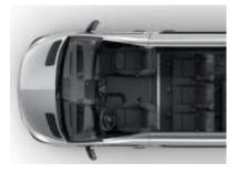
Three-seater bench in passenger compartment, **first** row, on left-hand side (in the direction of travel). All three seats are fitted with a three-point inertia-reel safety belts. ISOFIX child seat attachment points are on the two outer seats.
