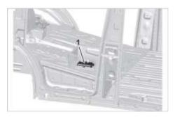
The main fuse box now contains four additional fuses (40/80/80/100 Amps) that are not utilized by the Sprinter and are dedicated fuses for electrical consumers on upfitted vehicles. Please look at the Sprinter operator's manual for more information on fuse locations.
