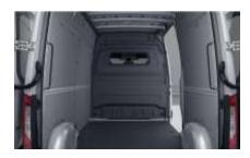
The full width sheet metal partition D51 with one plastic window located on the B-pillar is designed as one-piece for standard height roofs and two-pieces for high roof versions. These options now have a 0.59" (15 mm) deeper contouring at backrest height. This allows the front seats to be better adjusted to the driver and co-driver's comfort. The window dimension is 51.2" x13.4" (1300 mm x 340 mm) and is glued to the partition wall.
