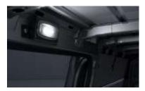
Two additional ceiling lights are fitted at the roof frame on the side wall. A door contact switch turns the lights on/off when the load compartment doors are opened/closed. The lights can also be switched on/off by the switch in the overhead control panel. In combination with code LC2, all standard ceiling lights in the load compartment come are LED.
