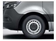
The vehicle is equipped with steel wheels painted arctic white (MB 9147).
