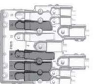
The main fuse box now contains four additional fuses (40/80/150/100 Amps) that are not utilized by the Sprinter and are dedicated fuses for electrical consumers on upfitted vehicles. Please look at the Sprinter operator's manual for more information on fuse locations.
