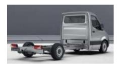
The Cab Chassis rear wall is fitted with a window of single-layer safety glass, size 52.4"x14.2" (1330 x 360 mm)
