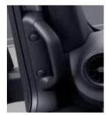
The grab handle is installed vertically on the driver and passenger door of the vehicle, and facilitates getting into the vehicle providing another option to hold on the way.
