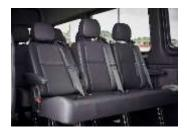
A three-seater <u>comfort</u> bench is fitted in the **first** row of the 14+1 passenger compartment. All three seats are fitted with a three-point seat belt and have additional seat bolster padding, allowing for enhanced seating comfort. This comfort variant can be equipped on Crew and Passenger Sprinters. Each row is individually reclinable as well as an individual recliner setting on each seat.
