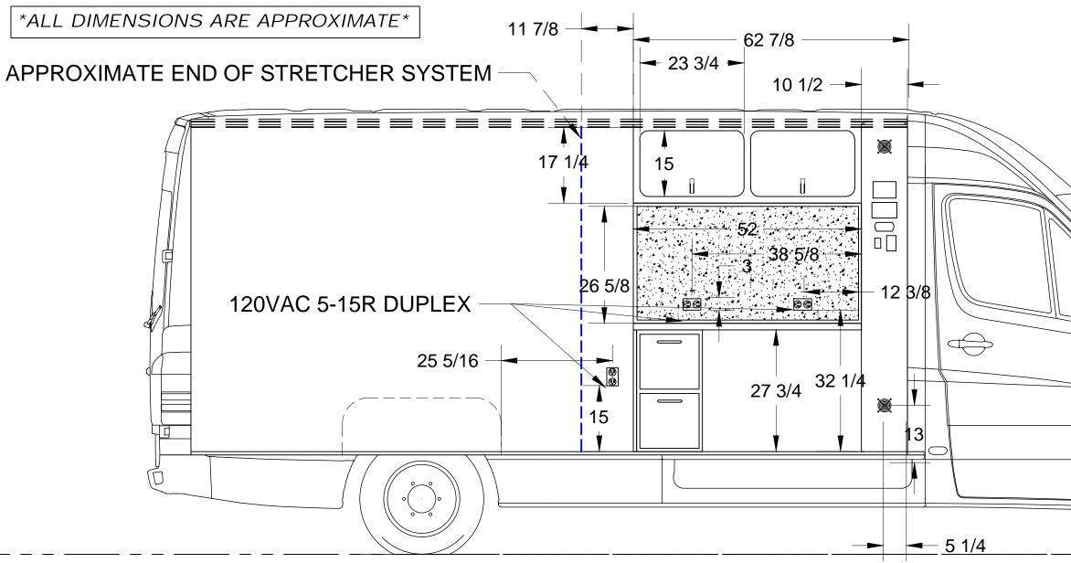
CREATE 2 LARGE ACCESS DOORS LOCATED ON THE SIDE OF THE ELECTRICAL CABINET FACING THE DESK. ONE DOOR BETWEEN D AND OVERHEAD CABINETS, AND ONE DOOR BELOW DESK.
