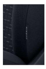
The thorax-pelvis sidebags are complete integrated in the back rest of the driver's and co-driver's seat. A tag located at the back rest's outside shows the installation of the sidebags. In a side impact, the side airbags can help to protect the torso and pelvis of the driver and co-driver. In addition they can stabilize the whole body to reduce the risk of serious injury in case of an accident.
