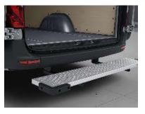
The code W75 includes a hot-dip-galvanized steel step fitted at the rear of the vehicle. The step measures  $63 \times 11,81$ " (1,600 x 300 mm) (width x depth). Solid rubber mouldings on the outer corners provide protection when manoeuvring.
