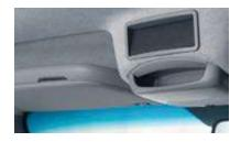
Green-tinted laminated safety glass with a darker tinting along the upper edge of the windscreen and a mounting plate for the interior mirror. The band filter reduces dazzle when the sun is low in the sky, but without impairing the driver´s view of the traffic. The mounting plate allows an easy retrofitting of the interior mirror.
