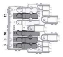
The main fuse box now contains 4 additional fuses (40/80/150/100 Amps) that are not utilized by the Sprinter and are dedicated fuses for electrical consumers on upfitted vehicles. Please look at the Sprinter operator's manual for more information on fuse locations.
