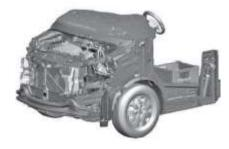
The cowl platform, is based on the cab chassis but without a wind-screen, roof frame, rear wall and doors. This type of vehicle provides upfitters a basis for fitting fully integrated superstructures e.g. campers or special-purpose solutions. The cowl version comes always without a driver and co-driver's airbag. Comfort seats with swivel base for driver and passenger are part of the vehicle configuration.
