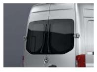
Water is supplied from the central washer fluid reservoir through flexible hoses to spray nozzles mounted in the wiper blades. The windows in the rear-end door provide a clear rear view, thanks to the wiper and washer system. If the front windscreen wipers are turned on, the rear window wipers are automatically switched on in addition when reverse gear is engaged or selected. The position of the wipers has changed from horizontal to vertical.
