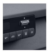
In addition to the heater booster, with the auxiliary hot-water heater, the departure time can be programmed in the instrument cluster using the stationary heater button in the climate control panel on the multi steering wheel.
