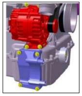
It is possible to attach an additional auxiliary alternator on the right side of the engine next to the oil pan, but this must be done using the factory option N62 as the bracket.
