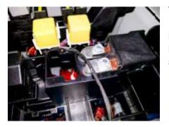
The relay is installed on the charge line to the auxiliary battery. It separates the starter battery consumers from the auxiliary battery consumers. When the engine is running, the relay allows both batteries to be charged (by the alternator) or discharged simultaneously.
