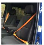
Orange safety belts replace the standard black safety belts for the driver and passenger (not with S23, twin passenger seat).
