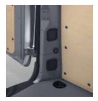
A 12-volt socket is located in the left-hand D-pillar trim of the passenger/cargo Van. The passenger Van also has a 12-volt socket in the right-hand D-pillar trim. Both sockets have a maximum power rating of 180 watts. Power can be drawn regardless of ignition key position. The sockets are supplied with power by the starter battery, except if code E2I/E2M is specified, in which case it is supplied by the auxiliary battery.
