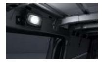
Two additional ceiling lights are fitted at the roof frame on the side wall. A door contact switch turns the lights on/off when the load compartment doors are opened/closed. The lights can also be switched on/off by the switch in the overhead control panel. In combination with code LC2, all standard ceiling lights in the load compartment come are LED.
