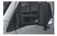
The standard exterior mirror is mounted on longer mirror arm and improves rearward visibility if an extra-wide body is fitted. Code FS2 is for a vehicle width of 90 - 92.9" (2190 - 2300 mm)
