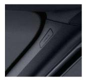
The window airbag units are installed along with the associated filling pipe at the inside of the respective roof frame behind the A-pillar paneling. The window airbags can protect the head area of the front passengers on the affected side in the event of a side impact. The code SJ3 deletes the codriver's window airbag. In this case only the driver's window airbag is installed. This allows special-purpose vehicles with modified passenger section.
