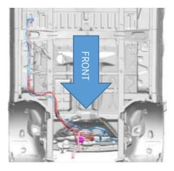
Two water lines (supply line/return line) are routed under the floor panel on the left-hand side of the vehicle, extending after the B-pillar. The ends of the two lines are connected by a hose. This allows an easier fitting of aux. heater exchanger from the accessories range. The opening in the floor (cargo/passenger van) /wooden floor for the warm air ducting and electrical parts e.g. climate control panel, wiring harness are not included.
