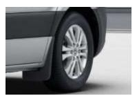
Plastic mud flaps are fitted to the wings behind the front wheels.
