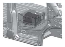
When ordering this, an absorbed glass mat (AGM) battery 12 V/92 Ah 850 A is installed into the passenger' seat frame. If an installation in the passenger's seat frame is not possible due to upfit restrictions, an additional 12 V / 70 Ah 720 A, AGM battery can be ordered into the engine compartment on the left hand side in driving direction, via code E2M. The battery is ideal for powering additional electrical consumers without putting a load on the starter battery.
