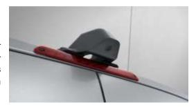
Trailer mode supports the driver when reversing to a trailer by zooming to the trailer hitch. To do so, special guide lines are shown in the display in addition to the pictures recorded by the reversing camera.
