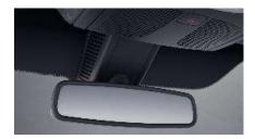
An interior mirror is attached to the front windshield to provide rearward visibility.
