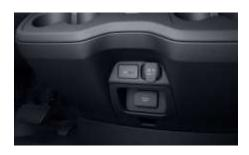
The 5-Volt USB-C power socket is located centrally in the lower part of the cockpit, below the center cup holder and next to the standard 12-Volt socket. Allows for these options to be within easy reach of driver and passenger.
