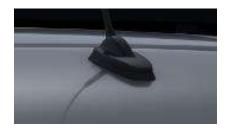
The antenna receives radio, telephone (up to 4G mobile phone signals), navigation signals and allows navigation and telematics systems to be fitted. If necessary, the aerial rod can be unscrewed when going through car washes. The number of available signals depends on the equipment installed in the vehicle – without telematics equipment or in conjunction with radio preparation (ERO) all 3 signals are available. In conjunction with MB audio sys-
