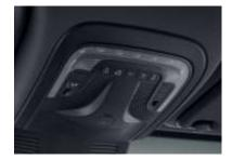
The Overhead Control Panel with interior lighting control, Code L1D, is comparable to the Comfort overhead control panel but includes an additional button to operate a retrofitted interior lighting for busses. The interior lighting in the rear is dimmed when activated.
