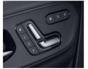
This electrical passenger seat is based on the driver's comfort seat code SB2 and has the same adjustment options. The main difference is the head restraint height and seat cushion length. All adjustments can be made electrically using the switches on the control unit located on the co-driver's door.
