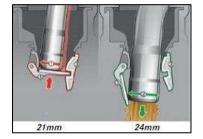
The protection system is designed for diesel models and includes a locking device with two levers that is made in such a way that it can only be unlocked by a standardized diesel pump nozzle. This prevents the tank from inadvertently being filled with gas. The diameter of the standardized gas pump nozzle (0.83" (21 mm)) is smaller than the diesel analogue (0.94" (24 mm)) and therefore too small to unlock the mechanism.
