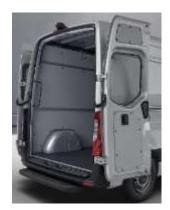
With W54, hinges are installed that allow the rear doors to be opened to the side wall of the vehicle. The new hinges hold the doors in place on its own without the need of rubber, magnetic bumpers on the door/side wall. This makes loading much easier in confined spaces, for example on ramps. The newly developed door hinges engage automatically at 90° and in the maximum opening position.
