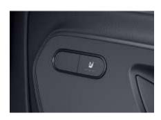
The heated seats are equipped with heating filaments in the seat cushion and backrest which are controlled by three-stage switches in the front door panels. When stage three is turned on for rapid heating, the system will run for approx. 7 minutes then automatically switches to stage two. After approx. 10 minutes, the seat heating automatically switches to stage one. The seat heating is automatically switched off after a further 20 minutes. It can be switched off manually at any time.
