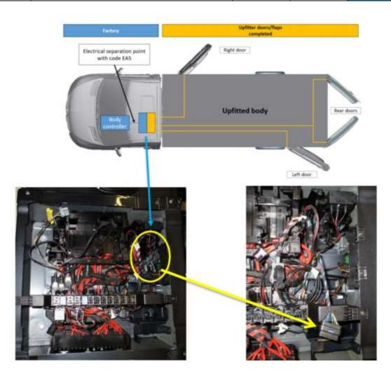
Pre-installation kit includes a wiring harness that gives cab chassis customers a chance to add additional aftermarket doors that use the same Mercedes-Benz key fob signal for unlocking and locking the doors and will also indicate door lock status in the instrument cluster.
