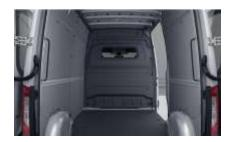
The full width sheet metal partition D51 with one plastic window located on the B-pillar is designed as one-piece for standard height roofs and two-pieces for high roof versions. These options now have a 0.59" (15 mm) deeper contouring at backrest height. This allows the front seats to be better adjusted to the driver and co-driver's comfort. The window dimension is 51.2" x13.4" (1300 mm x 340 mm) and is glued to the partition wall.
