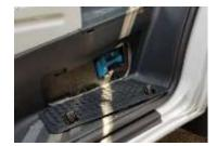
The hydraulic jack facilitates jacking up the vehicle to change a tire. It is located in a bracket in the entrance area on the passenger's side and is easy to remove.
