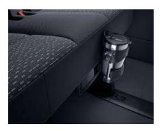
Cup holders are mounted between the rear seats on each bench. One cup holder can carry two cups or bottles with a diameter of up to 3.3" (84 mm). The cup holders can be ejected individually by pushing on its flap.
