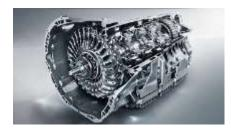
The Automatic Transmission 9G-TRONIC is fully electronically controlled with nine forward gears and one reverse gear. The gear ratios for the gear ranges are realized with planetary gear sets. All transmission functions and components are combined in one assembly module. The fully integrated transmission controller unit is located in the automatic transmission. This minimizes the number of interfaces to the vehicle wiring harness.
