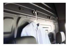
The two coat hooks in the cab are available for the cargo van and mounted above the head retrains on the partition wall inside of the driver's and co-driver's seats.
