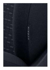
The thorax-pelvis sidebags are complete integrated in the back rest of the driver's and co-driver's seat. A tag located at the back rest's outside shows the installation of the sidebags. In a side impact, the side airbags can help to protect the torso and pelvis of the driver and co-driver. In addition they can stabilize the whole body to reduce the risk of serious injury in case of an accident.
