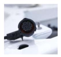
Wiring for trailer hitch that runs along the inside left frame. E40 includes a seven-pin connector and provides power for trailer lightning systems (tail lights, brake lights, direction indicators, rear fog lights and reversing light) and allows electrical operation. The trailer wiring is bundled up and temporarily attached to the frame during transport. This allows for installation of an authorized accessory trailer hitch by the body builder.
