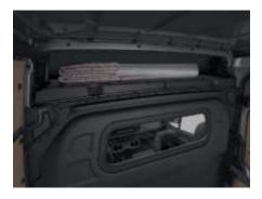
The storage compartment above the roof paneling uses the space between the headliner of the cab and the vehicle's high roof (D03) as an additional storage facility. The compartment is accessible from the loading area and can support a load up to 77 lbs. (35 kg).
