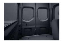
The luxury interior paneling, code V21, in dark grey fabric gives the passenger compartment a representative look, and also improves the noise and heat insulation. The paneling is made of wood-dust filled polypropylene boards and a 0.12" (3.05 mm) thick layer of polyurethane foam, all lined with fabric. This paneling includes 5V USB-C charging ports with a smart phone holder for each row installed on the left side of the vehicle.
