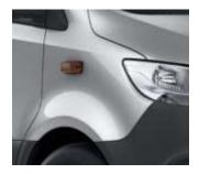
The direction indicators are mounted on the left and right front fender instead of on the outside mirrors.
