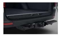
In conjunction with a trailer hitch Q24/QA2, it is possible to order a black painted step (7.48 x 20.47" (190 x 520 mm)) consisting of a tubular steel frame with a welded anti-slip tread surface. The step is bolted onto the right side of the trailer coupling and allows an easier entry and exit at the rear.
