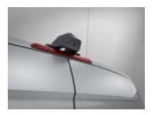
An additional LED brake light is fitted at the rear edge of the cargo van or passenger roof. The third brake light does not affect the height of the vehicle at the rear.
