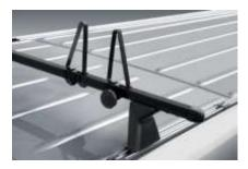
Two C-channel rails made of aluminium are permanently mounted in the lengthwise grooves on the vehicle roof. Maximum roof load (including basic carrier bars) 110 lbs. (50 kg) per crossbar. Maximum roof load for the standard roof is 660 lbs (300 kg) (six crossbars) and 330 lbs (150 kg) for the high roof (code D03) (three cross bars).
