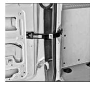
When loading and unloading on an incline or, for example, in strong winds: with the optionally available additional blocks, the open rear doors of your Sprinter are mechanically fixed at an angle of 90°. This facilitates access to the load compartment and ensures that the rear doors do not close unintended.
