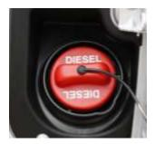
Instead of the standard black filler cap a red filler cap clearly labelled 'DIE-SEL' is mounted. The red color serves as an optical warning for the customer when refueling. This should prevent the customer from using the wrong type of fuel and having to pay for repairs.
