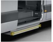
The electric step automatically extends when the sliding door opens, and retracts after the sliding door closes. This operation is possible without a use of the ignition key. The electric step is 47.24" (1200 mm) width and 11.42" (290 mm) depth. The maximum permissible capacity is 330 lbs. (150 kg). The aluminum step with a hot- dip galvanized cassette has a self-weight of 92 lbs. (42 kg).
