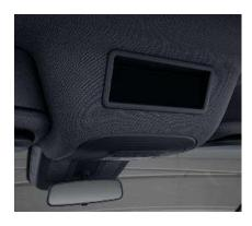
An opening (1 DIN slot) is centrally located in the headliner above the windshield. This slot can be used for additional electronic devices. It comes with a cover for delivery and includes a cable set which reaches into the slot and offer the following connections:
