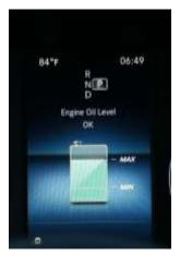
When parking the vehicle for a longer period of time, the last saved oil level is displayed at the start of the engine. The notification must be acknowledged by the driver. In addition, the oil fill level can be accessed via the service menu on the instrument cluster. It also scans a too low/high oil level in order to prevent engine damage.
