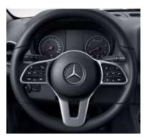
The leather steering wheel, comes with a 3-spoke design and is lined with 'nappa' leather and a perforated grip area. The standard matt black steering wheel cover is replaced by a silver chrome version.
