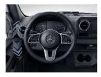
The steering wheel is manually adjustable for tilt and height. To provide a large adjustment range, the wheel can be tilted at a vertical angle between 28 and 32 degrees and adjustable axially by 2.36" (60 mm) and 1.96" (50 mm) in height. The adjustment is performed by a lever on the steering column.
