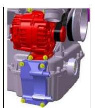
It is possible to attach an additional auxiliary alternator on the right side of the engine next to the oil pan, but this must be done using the factory option N63 as the bracket.
