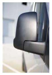
With code FU5, the exterior mirrors are fitted without turn signal indicators. Due to the omission of the indicators the mirror housing is not as wide, thereby overall width of the vehicle is reduced by approx. 0.78" (20 mm) each side. Other dimensions and the geometry of the mirror glass, also in combination with code FS2, extra-long mirror bracket, remain identical with those of the serial exterior mirrors. The mirror heating, code F68 as well as F64, is not available.
