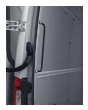
This grab handle(s) is installed vertically on the left D-pillar and allows an easier entry to the load compartment through the rear door.
