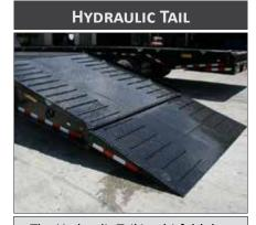
The Hydraulic Tail is a bi-fold that extends to allow easy loading of equipment with a very low load angle. In the transportation mode the flip under ramp folds into the beaver tail for a shorter overall trailer length.
