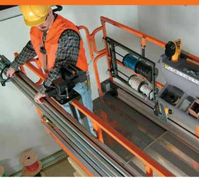
With our Plumber's Package, you have everything you need to get your plumbing work done more efficiently. Manufacturer-approved pipe racks provide positive retention of materials outside of the platform, helping prevent rail damage and optimizing platform space.
