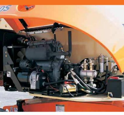
The JLG SkyPower<sup>®</sup> system delivers the power you need to conveniently operate other JLG accessories. With the SkyPower system on your machine, you get a 7500W generator with a power cable. Easily add and provide power to other JLG accessories, including SkyWelder<sup>®</sup> and SkyCutter<sup>®</sup> packages.
