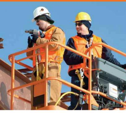
The SkyAir<sup>®</sup> onboard air compressor delivers 9.3 CFM of air at up to 125 psi—increasing productivity by reducing the risks, costs and hassles of tethering to a separate groundbased compressor.
