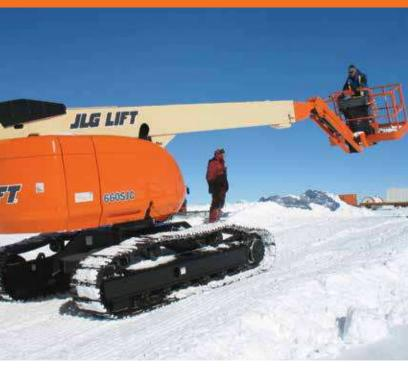
The JLG<sup>®</sup> Cold Weather Kit includes a battery blanket, hydraulic tank heater, block heater and glow plugs (diesel only).
