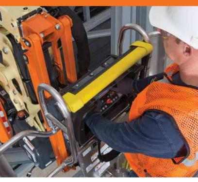
Boom lift operators experience enhanced control panel protection with this aftermarket accessory. When activated by approximately 50 lb (23kg) of force, SkyGuard<sup>®</sup> stops all functions in use at the time.
