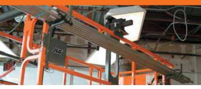
Conserve platform space and reduce trip hazards by storing the materials on the outside of the platform. Pipe racks help keep your tools and materials organized and within reach. Pipe racks come standard with Plumbing, Plant Maintenance and Electrician packages.
