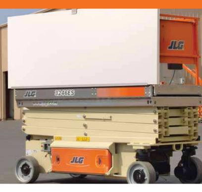
You don't need to clutter your platform with drywall, plywood or sheet rock. With the factory-approved panel carrier, you can load panels outside the rails in the carrier tray, where it's easier to transfer the panel to its elevated installation site.
