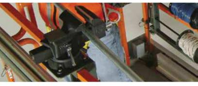
A factory-approved, rail-mounted 5  $\frac{1}{2}$  in. bench vise offers a convenient and safe method to securely hold material as you work with it—whether for threading and cutting or gripping other materials.
