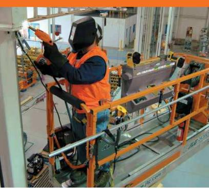
Ideal for spot welding, this self-contained wire-feed welder saves time by eliminating the need to move bulky tanks or cumbersome weld leads. The leads are integrated into the scissor lift; the scissor lift's batteries power the welder. It includes 15 ft (4.5 m) of cable, one spool of .035 in. (.09 cm) wire, four weld tips and a gas line.
