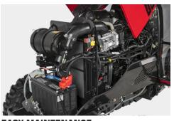
**EASY MAINTENANCE** Lift-up hood and side panels allows for easy access to battery, air filter, and fuel tank. Servicing your vehicle is as easy pushing a button.
