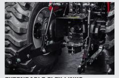
**EXTENDABLE FLEX LINKS** All 1600 series tractors have available extendable flex links (standard on 1635 & 1640) to adjust the 3-point and easily mount any implement.
