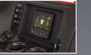
Automotive-style dash with 4.3 inch LCD instrument display highlighting speed, RPM, gear position, fuel level, battery voltage, engine temperature and oil change reminders
