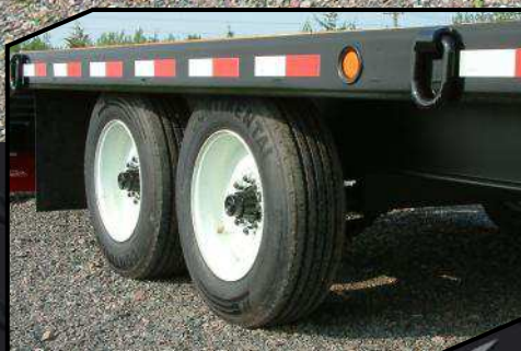
Single-wheel tandem axle. 8K Dexter Torflex axles with rubber-ride suspension.
