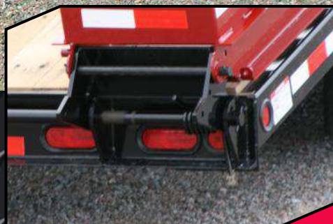
One-way spring-assist ramps and grommet mounted incandescent lights.
