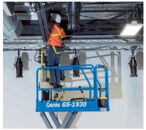
Attached to the platform rails, it enables operators to get into restricted spaces safely and increases productivity. This additional deck has a 225 lb (102 kg) capacity. When not in use it folds flat for storage.
