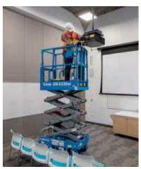
This scissor lift is equipped with an efficient, all-electric DC drive system that offers productive power for getting around indoor jobsites with quiet, zeroemissions operation. Heavy-duty and rental-ready, this new micro-sized scissor lift's top applications include construction in space restricted or congested locations, such as offices, high rise and retail spaces, as well as facility maintenance tasks.
