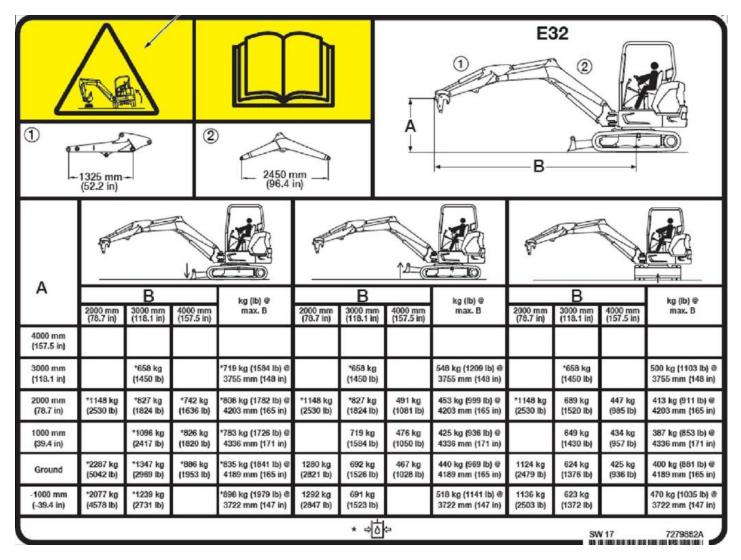
E32R Standard Arm, Heavy Counterweight Machine with canopy and rubber tracks, without bucket.
