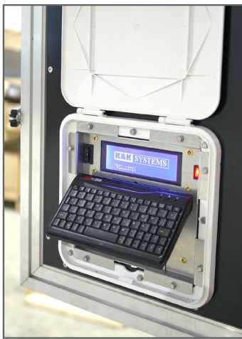
Onboard keyboard programming controller is built into the back of the display.
