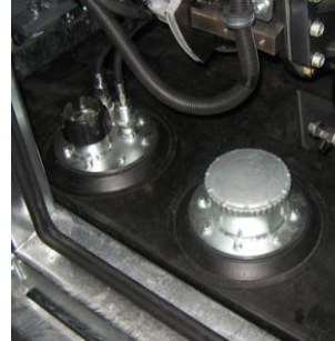
Fuel tank Double wall fuel containment, corrosion-free, 80 US Gallon, high-density polyethylene (HDPE) fuel tank, located in base of canopy.
