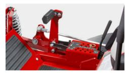
**Foot-Operated Deck Lift** With adjustable pedal, can change cut height in 1/4" increments from 1.75"- 5".
