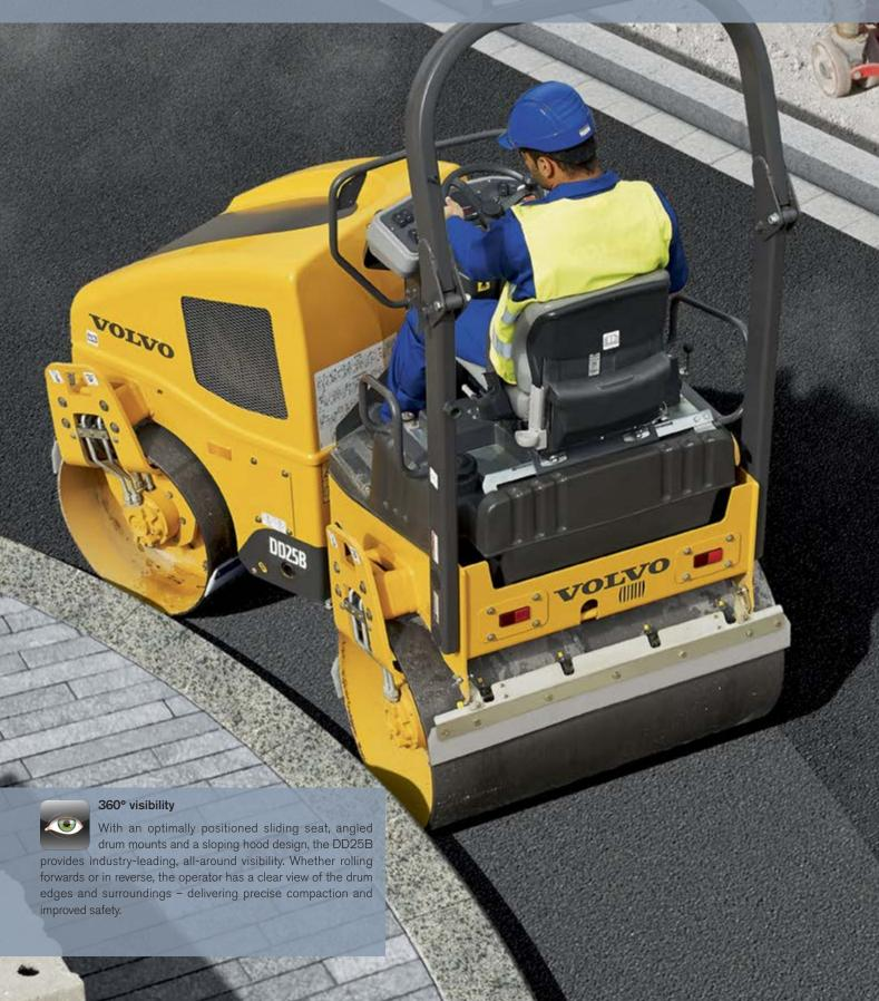
Introducing the DD25B, a highly efficient double drum compactor designed to increase performance and reduce fuel consumption on small scale compaction projects. Featuring the new Volvo D1.7A engine, this machine meets the strict Stage IV/ Tier 4 Final emissions regulations without adding an exhaust after-treatment system. Experience increased machine performance and enhanced productivity with Volvo.
