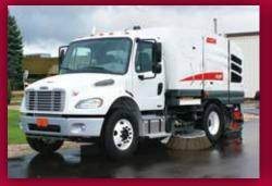
**CONVENTIONAL CHASSIS** Conventional chassis are built for sweeping and provide outstanding visibility, comfort, safety, and productivity. The short wheel base and unique steering geometry allow maximum maneuverability. A choice of Freightliner or International conventional chassis are also available.
