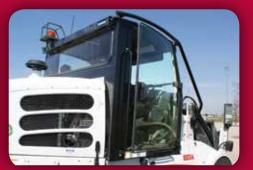
LIMB GUARD Heavy-duty guards surround cab and protect sweeper by guiding lowhanging tree limbs up and over the Pelican. Available in right hand, left hand, or dual configuration.
