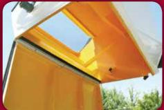
LIFELINER<sup>®</sup> HOPPER SYSTEM The LifeLiner system is a specially designed hopper liner and finish system that greatly improves the life, durability, and functionality of a sweeper hopper.
