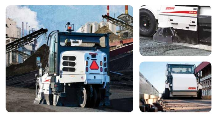
The Pelican with optional dry dust control maintains all the popular features and sweeping performance that have made the Pelican the best selling three-wheel sweeper–without the use of water for dust suppression. This means increased pick-up of fine particles over traditional, wet dust control sweepers, proven reliable year-round sweeping and significant water conservation.
